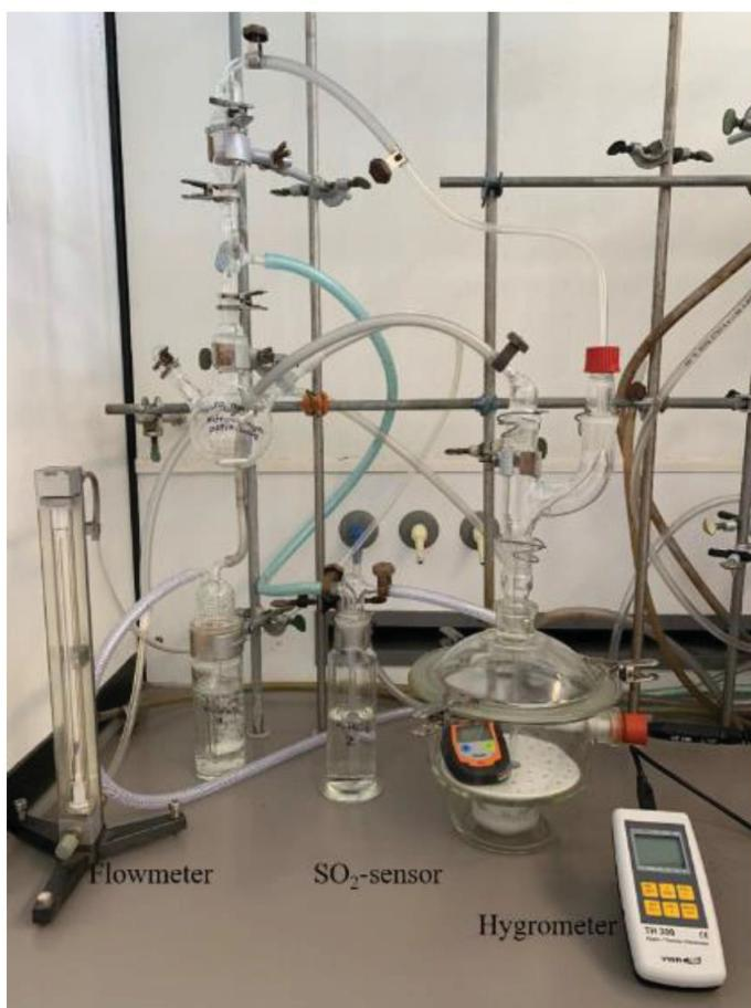
Figure S3. Setup for humid SO<sub>2</sub> exposure experiments.
