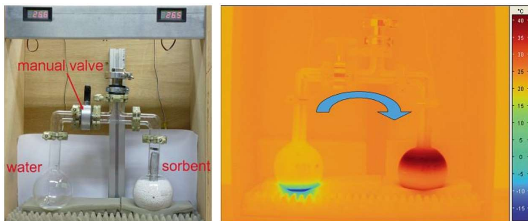
Figure 13: Experimental setup for the illustration of the working cycle in a TDC or AHP. Left: Picture of the apparatus before opening the manual valve. Right: Infrared photograph after opening the manual valve, indicating temperatures of T < -5\text{ }^{\circ}\text{C} in the water reservoir and T > 40\text{ }^{\circ}\text{C} in the sorption material. Reprinted from ref. 161 with permission, © 2013, Schweizerische Chemische Gesellschaft.
