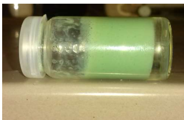
Figure 17: Stable nano-MIL-101(Cr)@HIPE from a water/cyclohexane mixture in a glass vial. After formation of the HIPE the glass vial was laid and kept structurally stable for at least 12 h.
