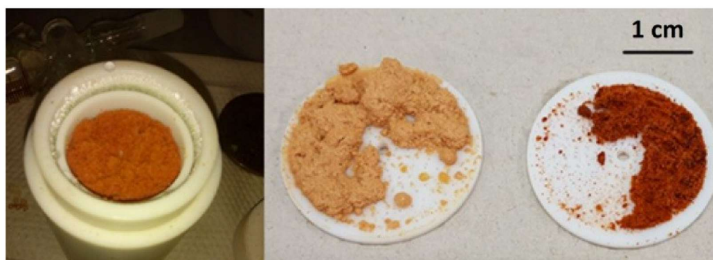
Figure S3 Left: Autoclave with DGC sieve, with MIL-100(Fe) product on top. Right: Products obtained from Fe(NO 3 ) 3 ·9H 2 O (left), FeCl 3 ·6H 2 O (right).
