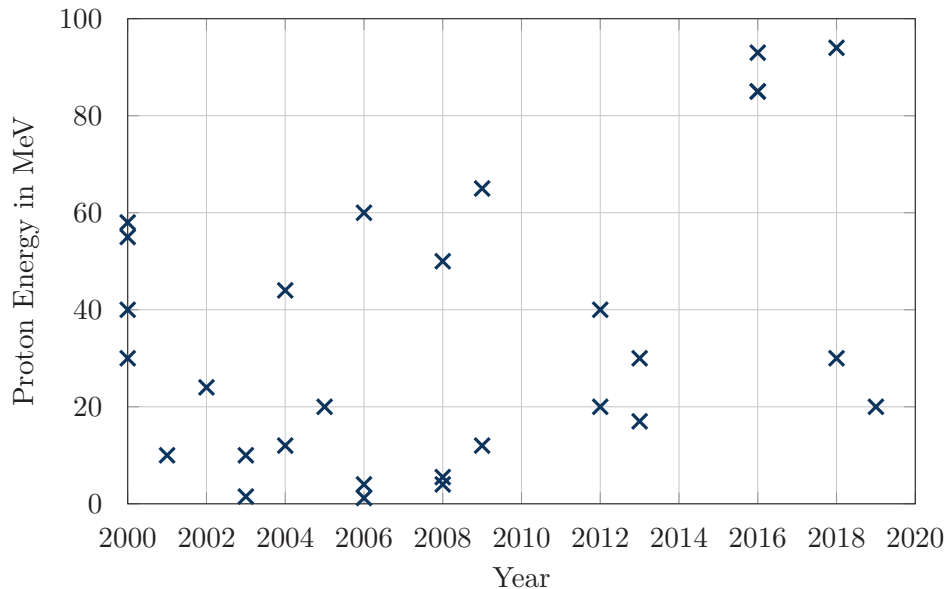
Figure 3.2: Development and status of laser-driven proton acceleration making use of quasi-static field and/or thin target foils (cf. App. A).
