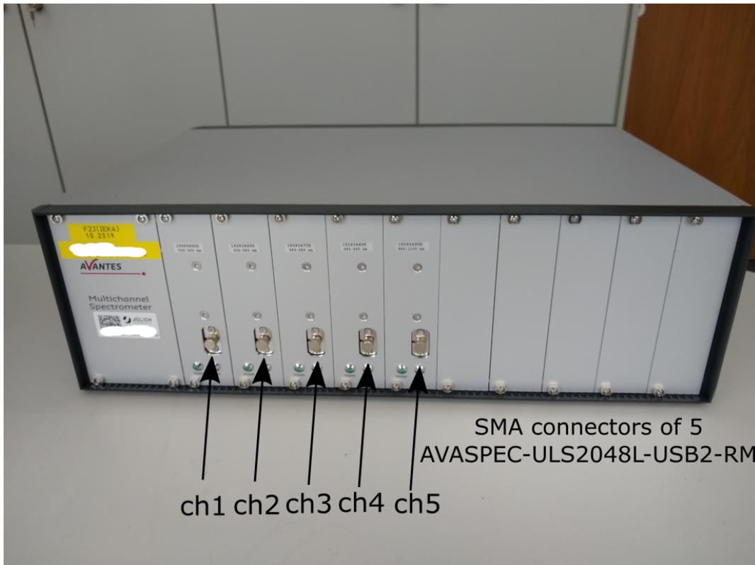
**Figure 2.14:** Desktop mount of 5 Avantes AVASPEC-ULC2048L-USB2-RM spectrometers with the power supply and the USB2 hub. Arrows point at the 5 SMA connectors for each channel (spectrometer). 5 free slots could be used for additional spectrometers.
