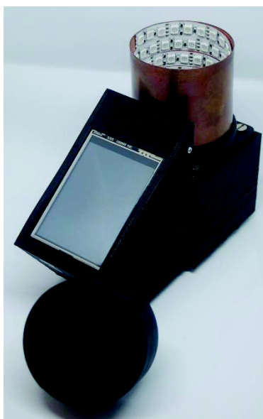
Figure 15: Photoreactor with LCD-display.
