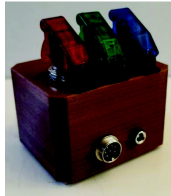
Figure 12: Controller using coloured switches.
