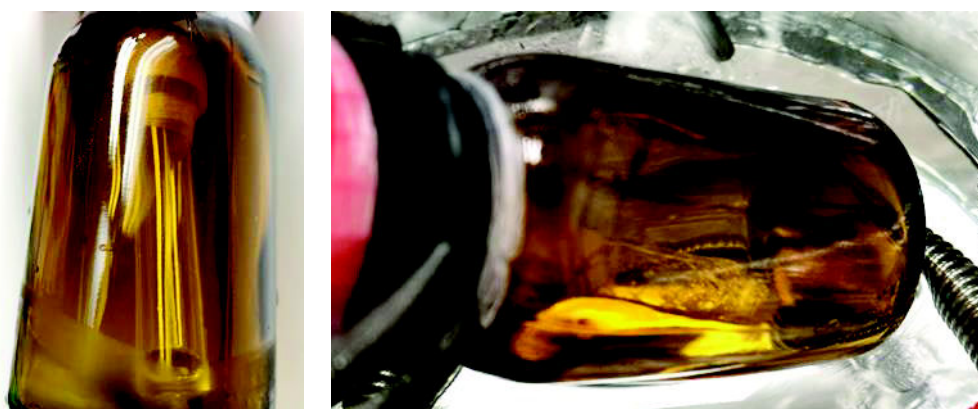
Figure 22: Sealed vial of {}^t\text{Bu}_3\text{P} 186 and \text{C}_4\text{F}_9\text{I} 101 inside a closed bottle under \text{N}_2 -atmosphere (left) and cooled to -7\text{ }^\circ\text{C} - -10\text{ }^\circ\text{C} inside a cooling bath (right).
