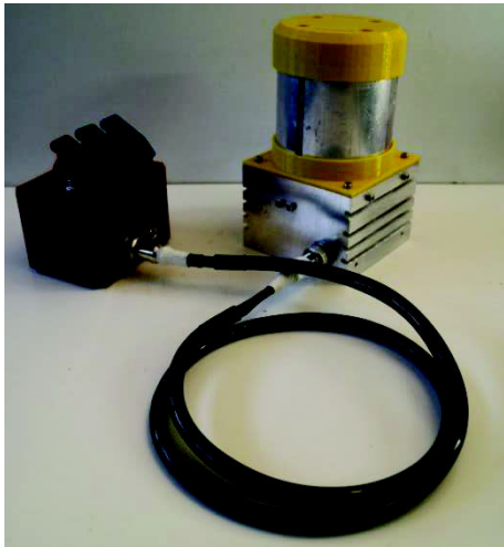
Figure 13: Combination of the photoreactor and the controller.
