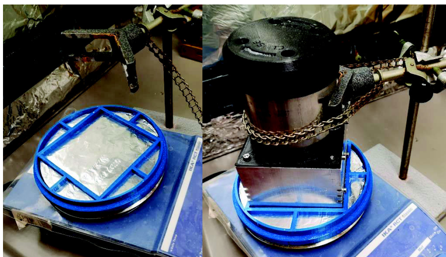
Figure 7: Centering support for the photoreactor on top of the magnetic stir plate (left) and with the attached photoreactor (right).
