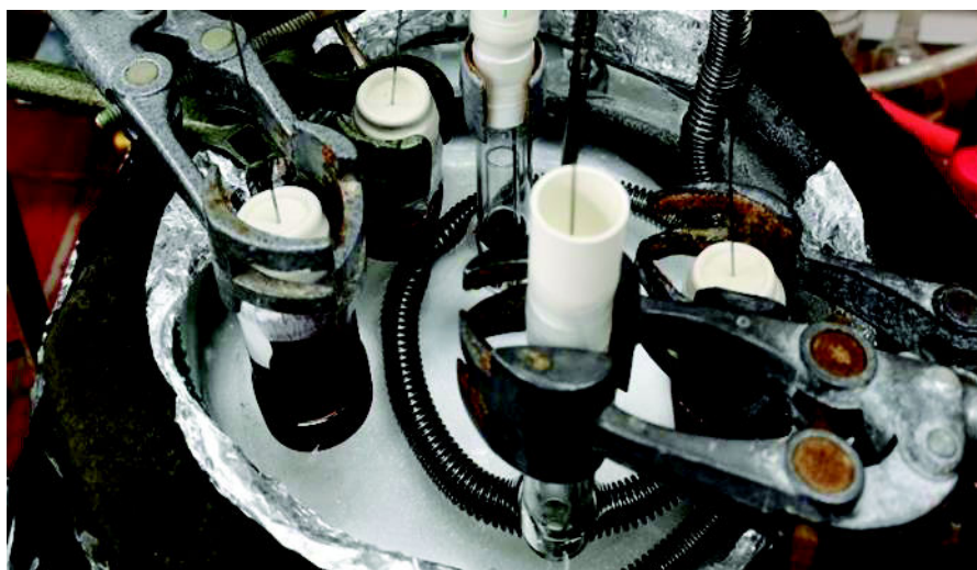
Figure 23: Sealed vials of t\text{Bu}_3\text{P} 186 , \text{C}_4\text{F}_9\text{I} 101 and a solvent inside a closed bottle under \text{N}_2 -atmosphere and cooled to -7\text{ }^\circ\text{C} - -10\text{ }^\circ\text{C} inside a cooling bath.
