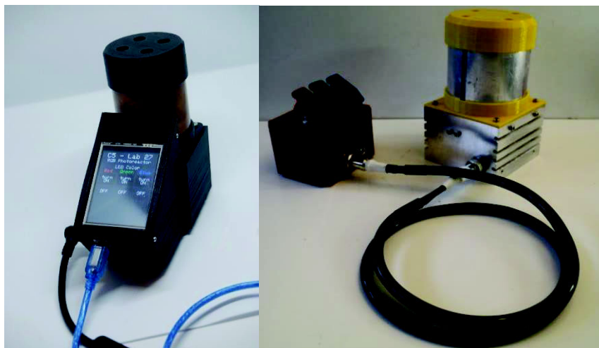
Figure 4: Self-designed photoreactors. With LCD display (left) and with manual light control (right). [4]
