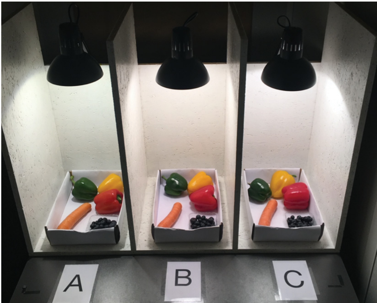
Figure 2. Depicted is the experimental setup for the pleasantness, naturalness and purchase preference ranking of the light sources used in Experiment 1 (halogen, LED80, BLED96) and Experiment 2 (halogen, LED80, VLED97). Each light source was installed in one of three identically build adjacent boxes. The assignment of the light sources to the boxes was balanced and changed on every day of the data acquisition period. A portable white platter filled with natural objects (blueberries, green pepper, yellow pepper, carrot and red pepper) was placed under the light sources. Note that in Experiment 1 there was only one portable white platter with natural objects instead of three identical white platters as in Experiment 2.
