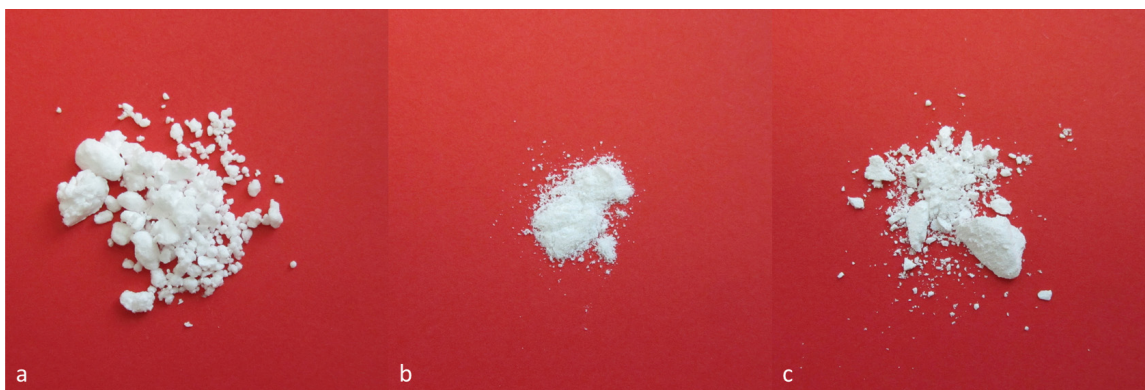
Figure 2.1. Freeze-dried Car-Asp at 1:1 molar ratio (a), melt-quenched carvedilol (b) and ball-milled Car-Asp at 1:1 molar ratio (c).
