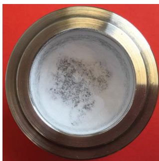
Figure 2.2. Milling jar containing ball-milled Car-Asp at 1:1 molar ratio.
