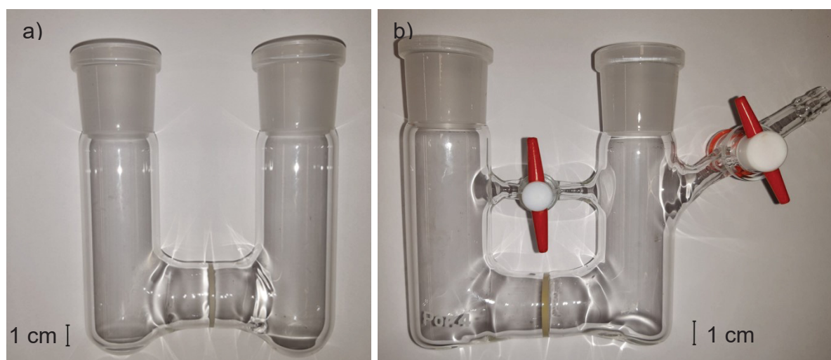
Figure 10: Picture of divided cell A , standard (a) and with Schlenk connections (b).
