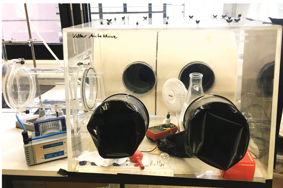
Figure 4.8: Home made glove box for cultivation of bacteria.
