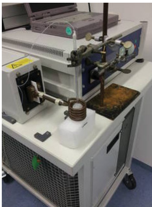
Figure 4.14: Oscillating electromagnetic alternating field (OEMF) or AC magnetic field: The image is taken from Physical - Chemistry Institute, University of Cologne where the measurements were carried out
