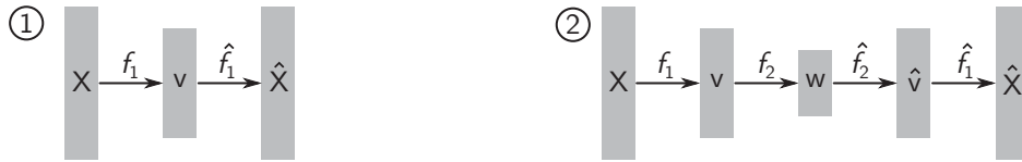
Figure 3.6: Two-layer stacked autoencoder. (1) A stacked autoencoder is trained by first training the outer encoder-decoder layers f_1 and \hat{f}_1 to reconstruct inputs X . (2) Then, the inner encoder-decoder pair f_2 and \hat{f}_2 is trained to reconstruct the latent feature representation v = f_1(X) of the encoder f_1 .
