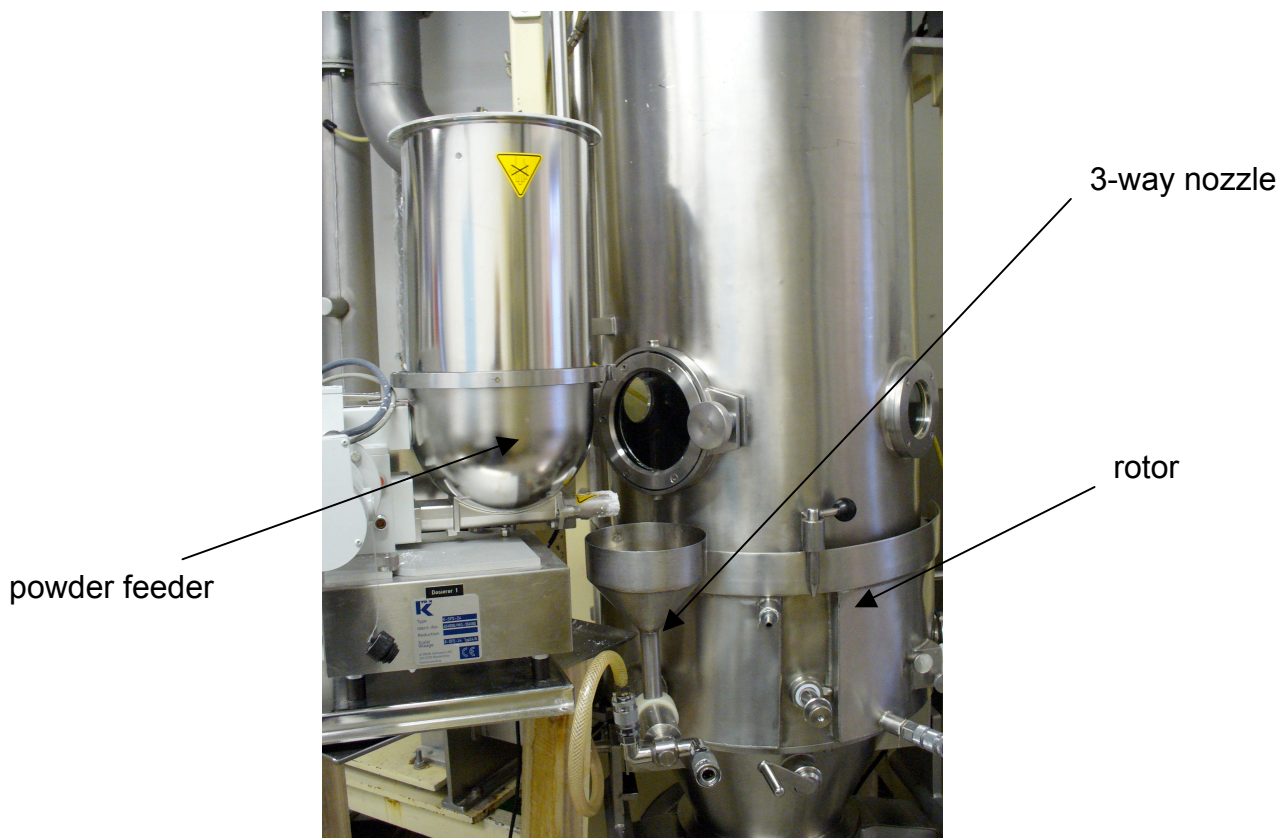
Figure 64: GPCG 5 with the gravimetrically powder feeder and the 3-way nozzle
