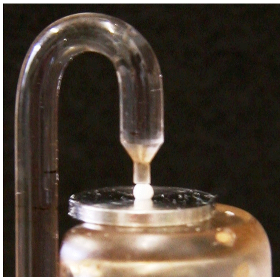
Figure 57: TMA sample holder designed to measure the film's glass transition temperature in situ
