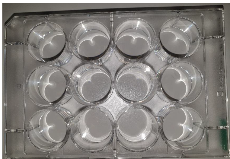
Fig. S3. Multiwell plate with 12 measuring chambers. The reader moves the plate in order to measure five points in each well.
