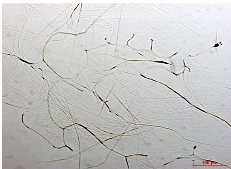
Figure 6-28 Optical microscopy image of the ternary system \text{H}_2\text{O} -LAS-DBC with a gellant concentration of 6.69 mM and a surfactant concentration of 20.09 mM. The sample was transferred onto the slide at 353 K and was allowed to cool to 298 K. The image was taken after 180 minutes (scale bar = 100 \mu\text{m} ).
