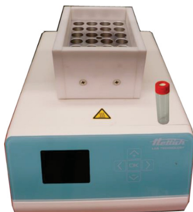
Figure 5-8 Illustration of the thermomixer from the company Hettich Benelux and the vial consisting of a pressure relief cap from the company Dunn Labortechnik GmbH.
