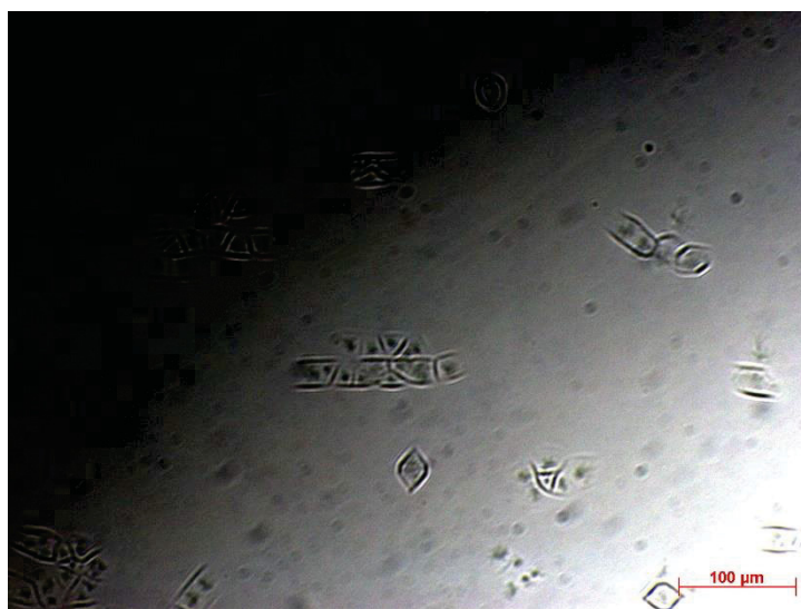
Figure 6-57 Optical microscopy image of the ternary system H 2 O-LAS-L-Tyr-L-Tyr with a gellant concentration of 6.69 mM and a surfactant concentration of 0.29 mM. The sample was transferred onto the slide at 353 K and was allowed to cool to 298 K. The image was taken after 20 minutes (scale bar = 100 \mu\text{m} ).
