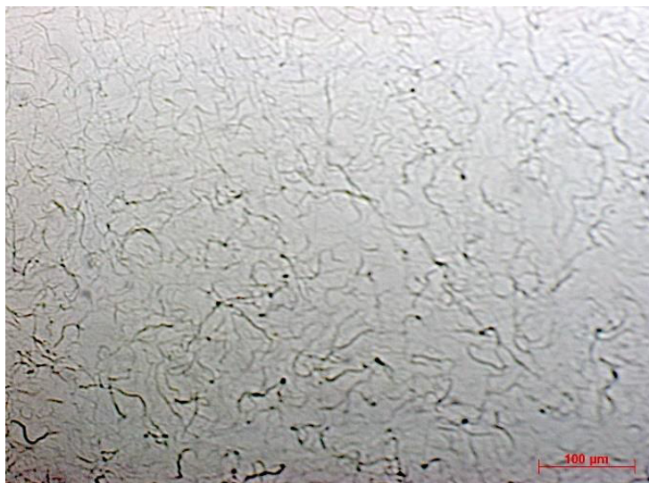
Figure 6-14 Optical microscopy image of the 6.69 mM binary system of H 2 O-DBC. The sample was transferred onto the slide at 353 K and was allowed to cool to 298 K. The image was taken after 20 minutes (scale bar = 100 \mu\text{m} ).
