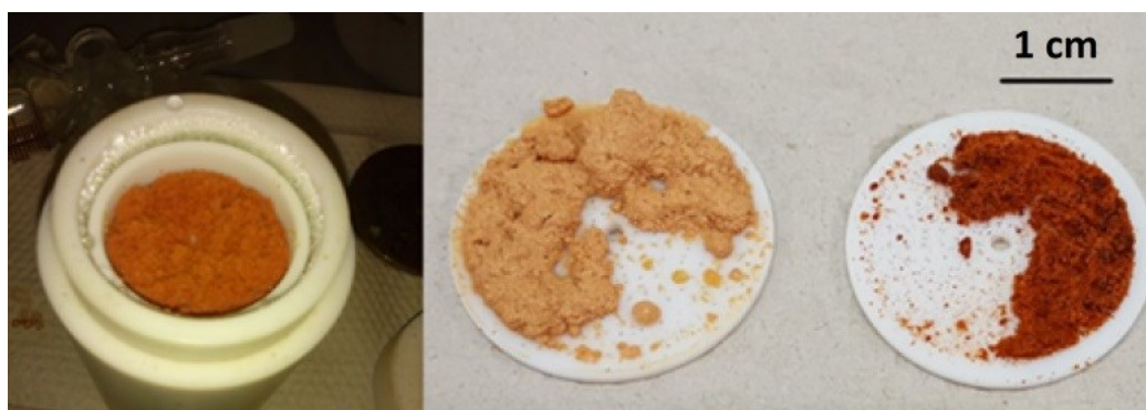
Figure S3 Left: Autoclave with DGC sieve, with MIL-100(Fe) product on top. Right: Products obtained from \text{Fe}(\text{NO}_3)_3 \cdot 9\text{H}_2\text{O} (left), \text{FeCl}_3 \cdot 6\text{H}_2\text{O} (right).
