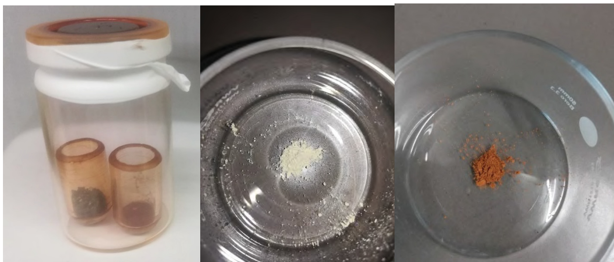
Fig. S11 Photographs of the set up for iodine adsorption (left), Ce-HHU-1 before iodine adsorption (middle) and after iodine loading (right).
