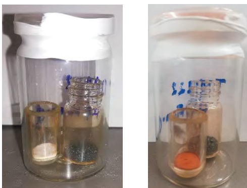
Figure S20. Pictures of the set-up of iodine adsorption for Hf-HHU-2, at the beginning of the experiment (left) and after some days (right).
