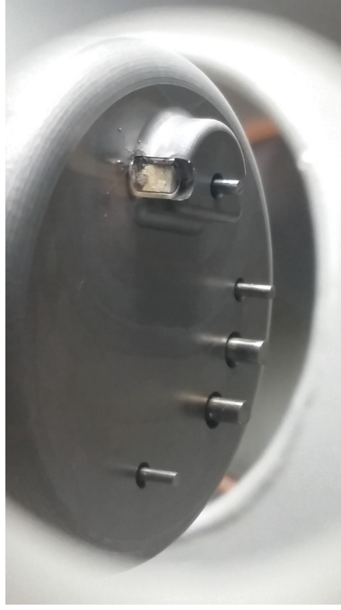
Figure 3.1: Superficial damage on pin 7 after the arcing.
