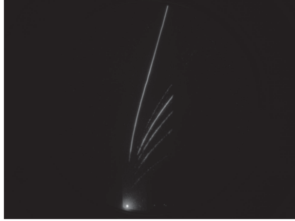
Figure 6.2 – Picture taken from the 0^\circ MCP on a typical two beam shot. In the lower part the zero point due to x-ray radiation can be seen. Different parabola-like traces indicate different ion species depending on their charge to mass ratio. Closer proximity to the zero point indicates a higher particle energy.
