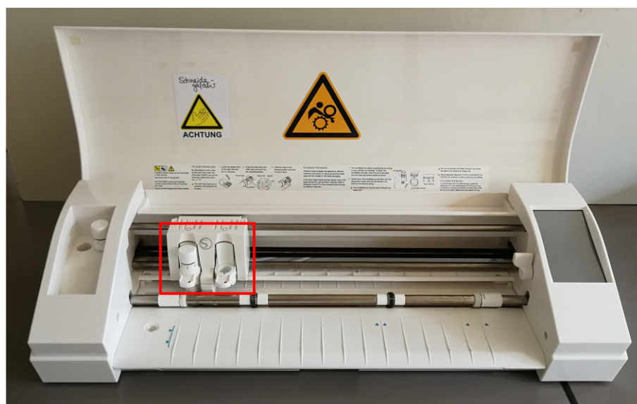
Figure 60: Cameo ® 3 cutting plotter with movable cutting unit (marked in red).
