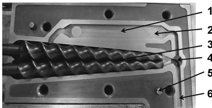
Figure 5. Open barrel of a micro-conical twin-screw extruder (HAAKE MiniLab): backflow channel (1), pressure probe (2), conical screws (3), bypass valve (4), temperature probe (5), extrusion channel (6) (adopted from [63], by courtesy of Elsevier).
