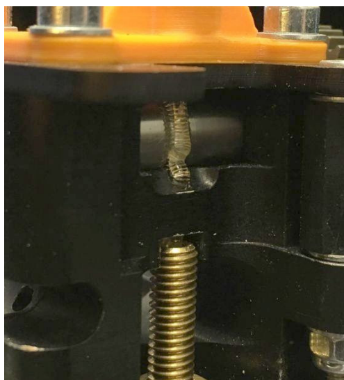
Figure 25. Unclosed print head with F16 filament showing plastic deformation due to frictional heat.
