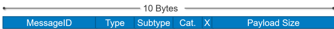
Figure 4. Message header. Cat.: message, request or response; X: exclusive or not (ordering).
