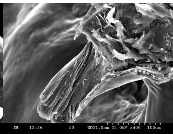
Abb. 23: ICBM, coating: PLGA 5% in DMSO, 400x
