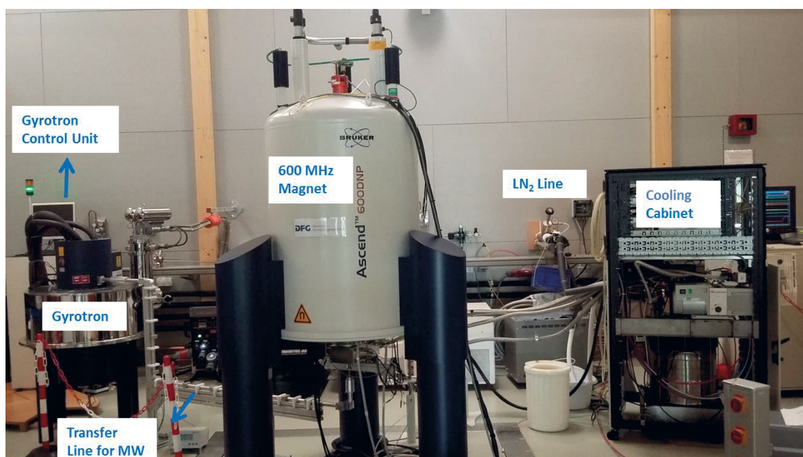
Figure 5. A commercial Bruker Avance III HD spectrometer operating at 600 MHz, equipped with a 395.18 GHz second-harmonic gyrotron, corrugated wave guide and cooling cabinet. It is located at the Jülich-Düsseldorf Biomolecular NMR Center in Jülich, Germany and jointly run by the Forschungszentrum Jülich and the Heinrich-Heine-University Düsseldorf.
