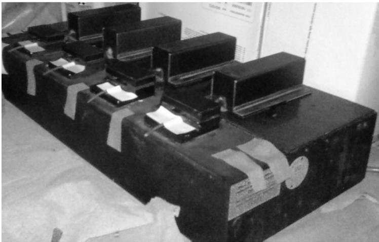
**Fig. 2.4:** Equipment for measuring blood pressure and heart rate using tail-cuff method. Four mice are sitting in a black box each, their tails are visible.
