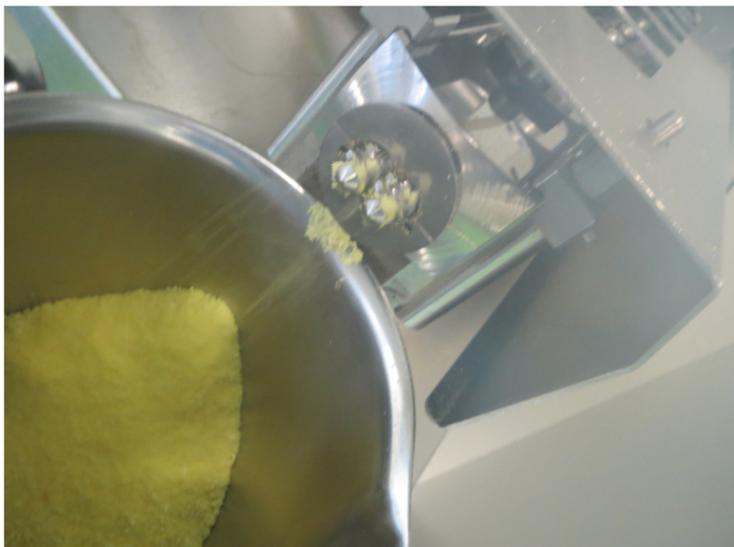
Figure 37: The in-barrel-drying process for lumefantrine. Water was evaporated via the opening at the TSG exit.
