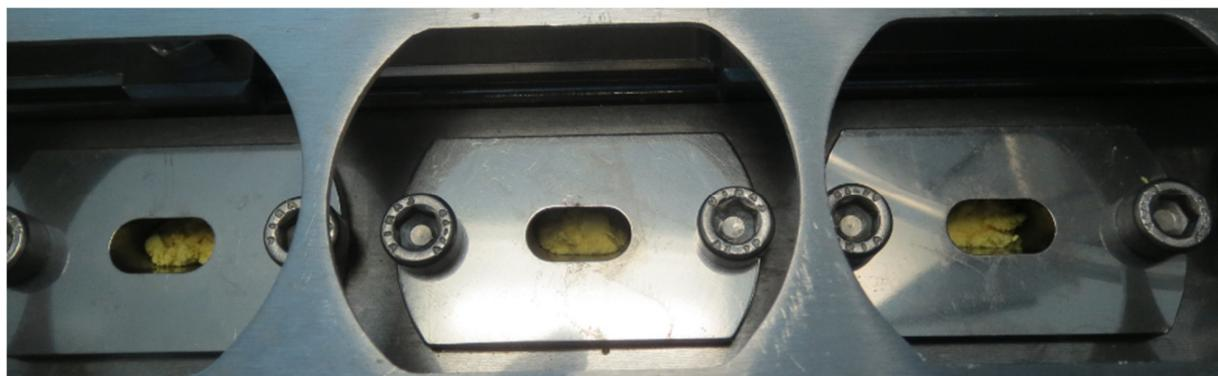
Figure 34: Material accumulation in the degassing vent ports. Over time ports got clogged and evaporation of water failed.
