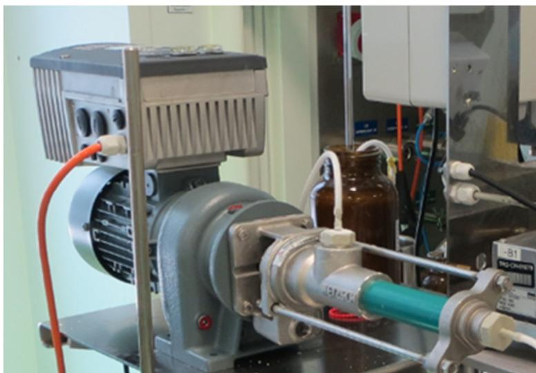
Figure 8: Setup of the progressing cavity pump.
