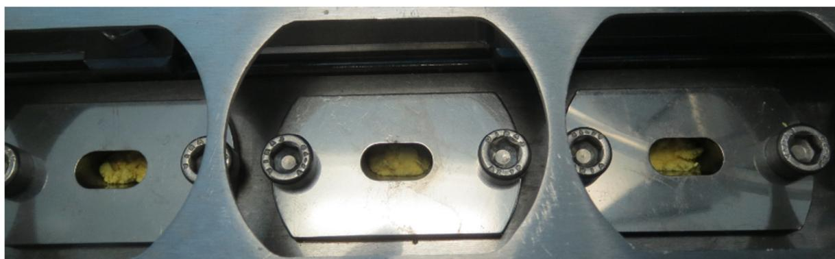
Figure 34: Material accumulation in the degassing vent ports. Over time ports got clogged and evaporation of water failed.
