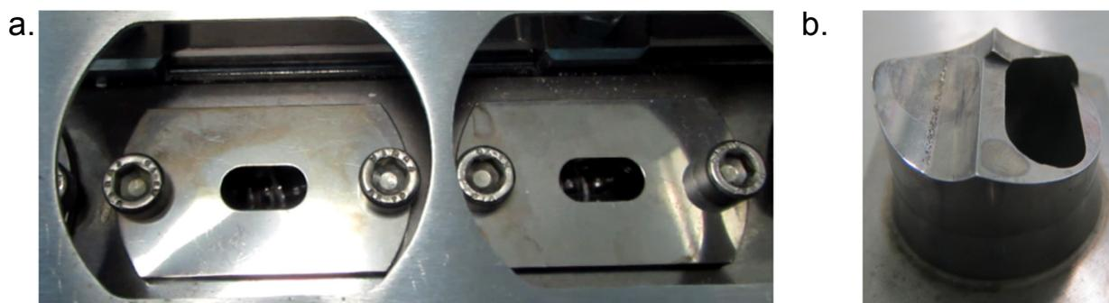
Figure 33: (a) Degassing vent ports, installed on the upper barrel in the zone of evaporation. (b) Bottom-view of a degassing vent port.
