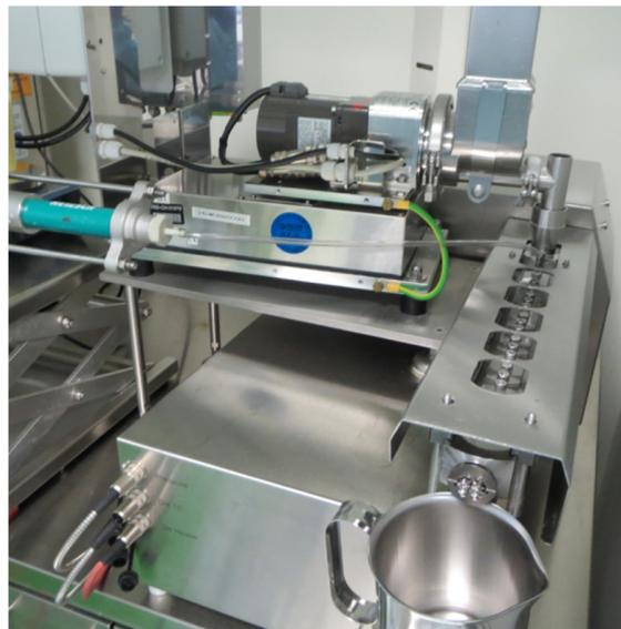
Figure 5: Process setup for the comparison of twin-screw wet granulation with API suspension feed and API dry blend feed. The solid (API blend or excipients blend) was fed using a twin-screw loss-in-weight powder feeder. The liquid (API suspension, suspending agent solution, or pure water) was fed using a progressing cavity pump.
