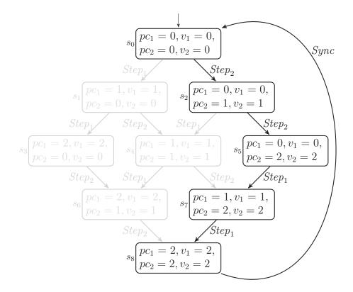
Figure 4.2.: State space of the *SyncThreads* model for n = 2
