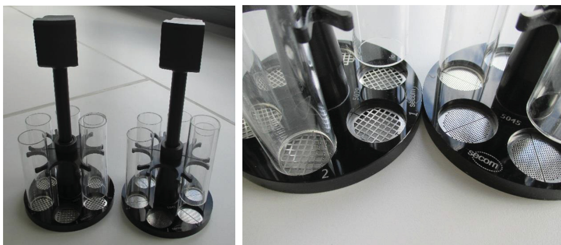
Figure 71. Disintegration baskets for the DisiTest 50 with 10 (left) and 40 (right) mesh.
