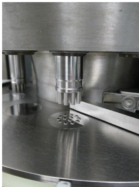
Figure 70. Biconcave 13-tip tableting tools for 3 mm mini-tablets.
