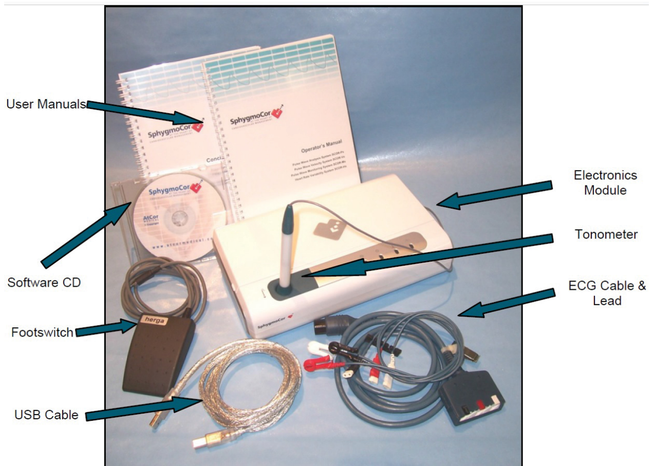
Figure 10: SphygmoCor with accessories (AtCor Medical Pty. Ltd. Sydney Australia 2010).
