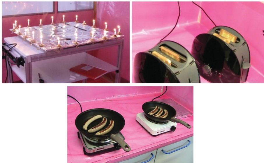
Figure 8: The activated exposure sources candles burning, toasting bread and frying sausages.
