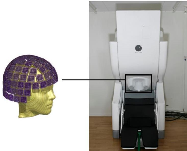
**Figure 2: MEG system.** Frontal view of the 306-channel whole-head MEG system (Elekta Neuromag, Helsinki, Finland) at the Institute of Clinical Neuroscience and Medical Psychology, Heinrich-Heine-University Düsseldorf. The insert on the left-hand side adapted and modified from Hari and Kujala (2009) depicts the MEG sensors (so-called SQUIDs) arranged within a helmet-shaped inlay.
