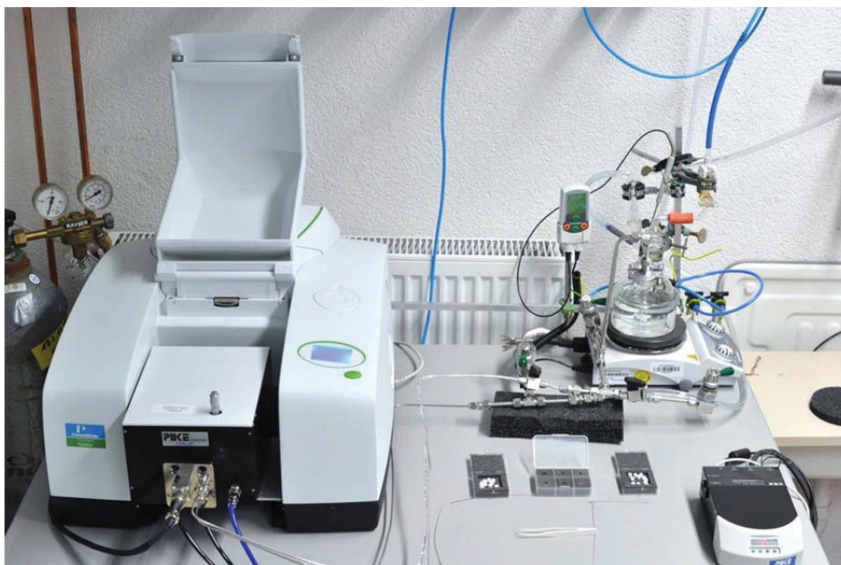
Figure 14 “Frontier MIR Performance System” equipped with “Frontier Diffuse IR” and “DiffusIR Env Chamber,900C” as well as a water reservoir for humidifying the gas stream.
