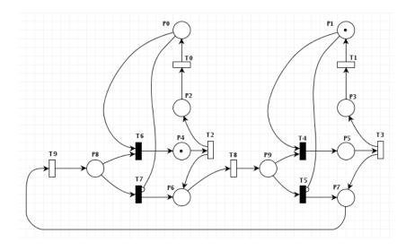
Figure 2.15.: Petri net graphical notation created with [DKS09]
