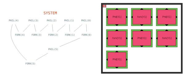
Figure 2.14.: Process communication visualization in FDR3 (left side) and TAPAs (right side) for the dining philosophers problem
