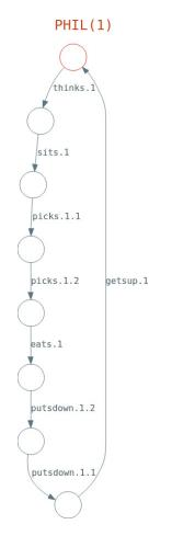
Figure 2.12.: Process visualization in FDR3 for PHIL(1) process of dining philosophers problem specification
