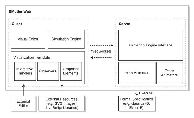
Figure 4.2.: Architecture of BMotionWeb
