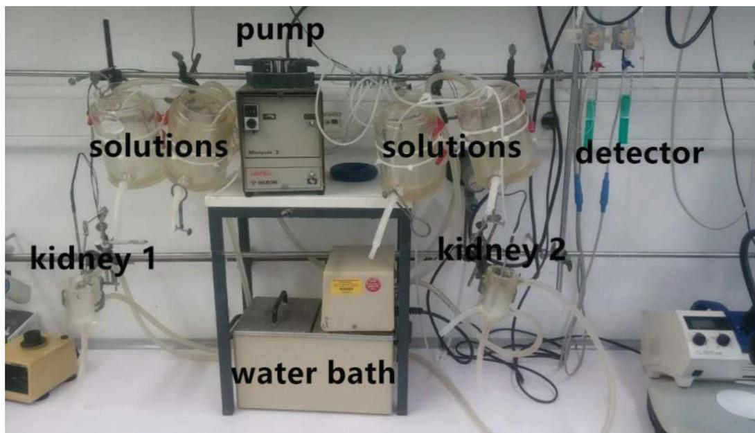
Figure 10 Isolated perfused kidney detector.
