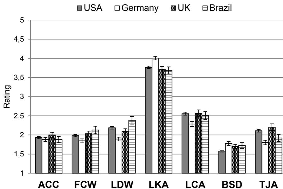
Legend: ACC: adaptive cruise control; FCW: forward collision warning; LDW: lane departure warning; LKA: lane keeping aid; LCA: lane centering aid; BSD: blind spot detection; TJA: traffic jam assist
