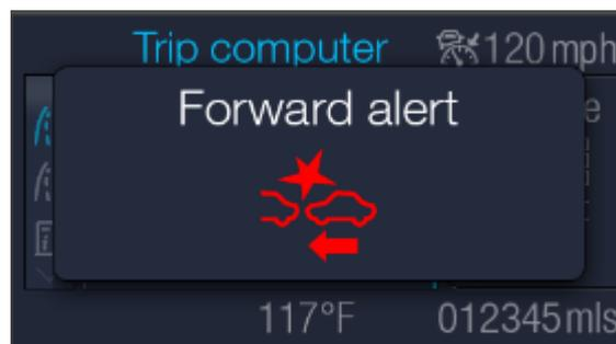
*Figure 3: Ford forward collision warning visual alert (Source: Ford)*
