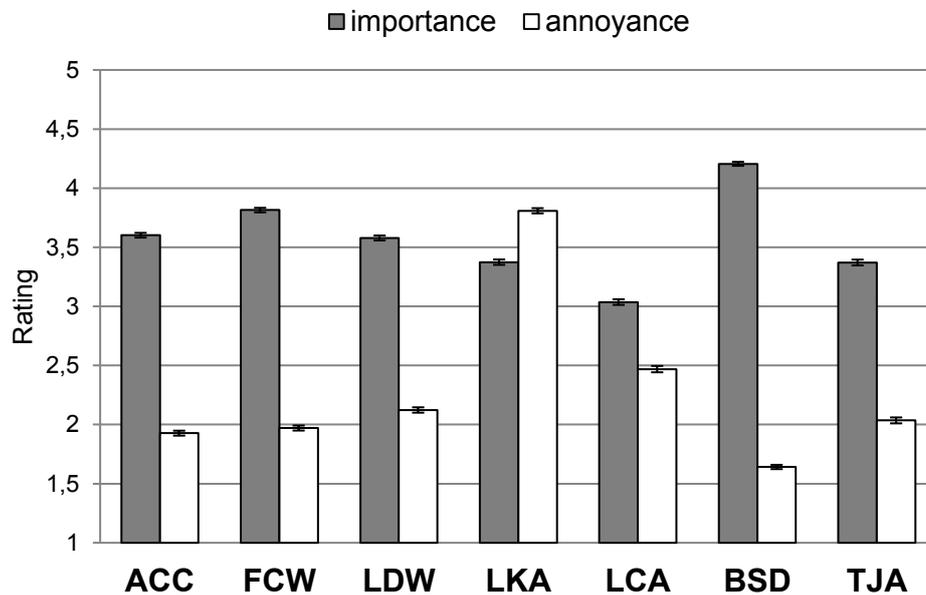
Legend: ACC: adaptive cruise control; FCW: forward collision warning; LDW: lane departure warning; LKA: lane keeping aid; LCA: lane centering aid; BSD: blind spot detection; TJA: traffic jam assist
