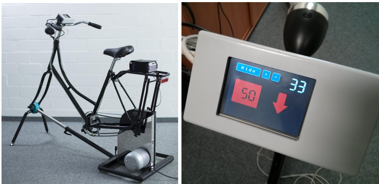
Figure 1. The BrainCycles experimental setup; left - classic Dutch frame and EEG amplifier mounted on the Cyclus2 ergometer; right - handlebar display presenting information about the current and the desired target cadence in rpm
