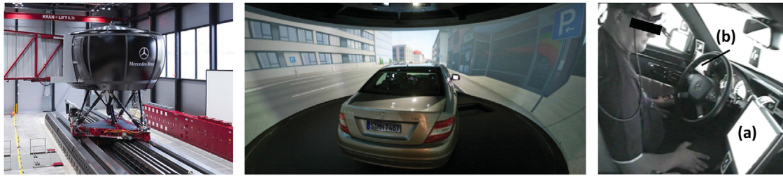
Fig. 1. Left: Mercedes-Benz driving simulator. Middle: Example of the inside of the simulator cell with a C-Class. Right: Vehicle interior with the touch screen used for secondary tasks (a) and the system status display (b).
