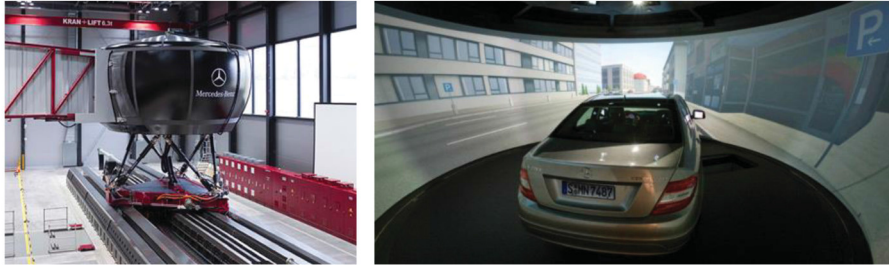
Figure 1. Mercedes-Benz driving simulator (left) and an example of the inside of the simulator cell with a C-Class (right).
