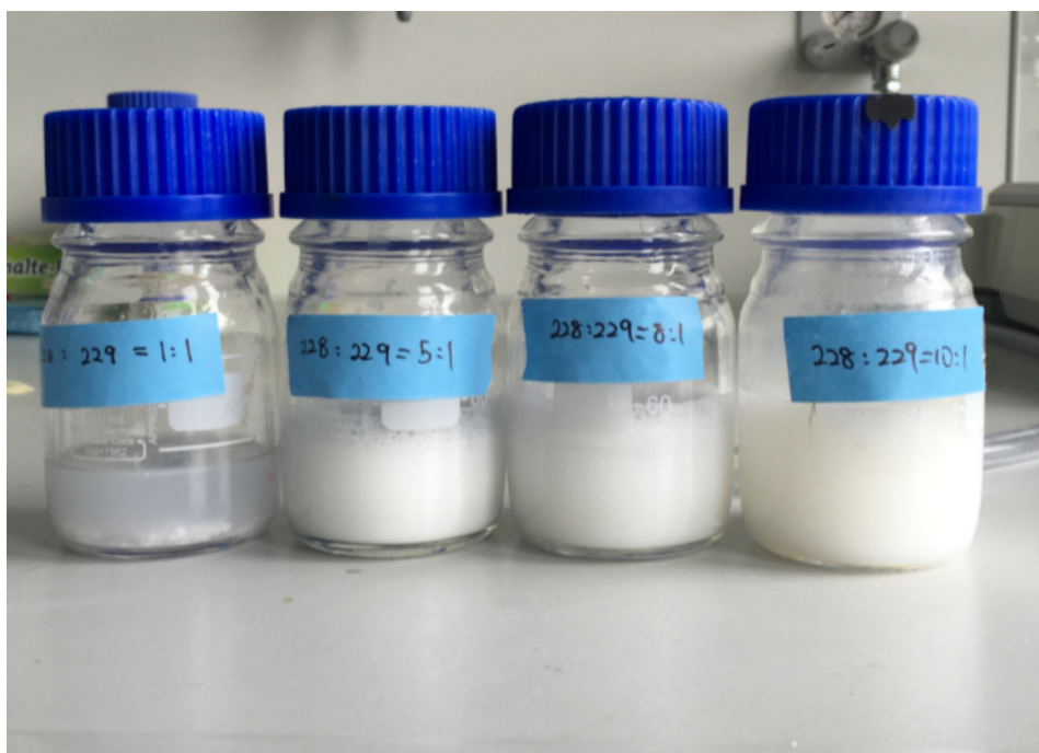
Figure 6.7: Dispersions of 228-229 at various weight ratios of amphiphilic 228 over hydrophobic 229. From left to right: m(228):m(229) = 1:1, 5:1, 8:1, 10:1 .
