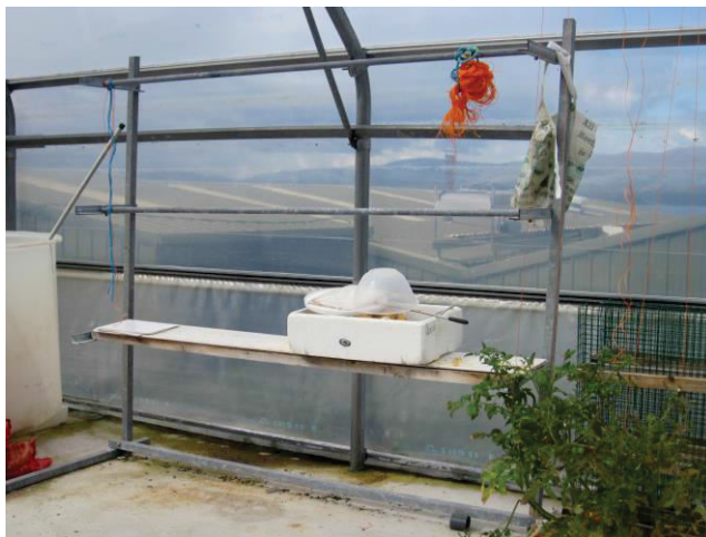
Figure 8: Photograph of the outdoor culturing frame. An outdoor replica of the culturing frame used to hang the bags was built for outdoor experimentation. The culturing frame was placed in the poly tunnel and an air supply system identical to the indoor system implemented.
