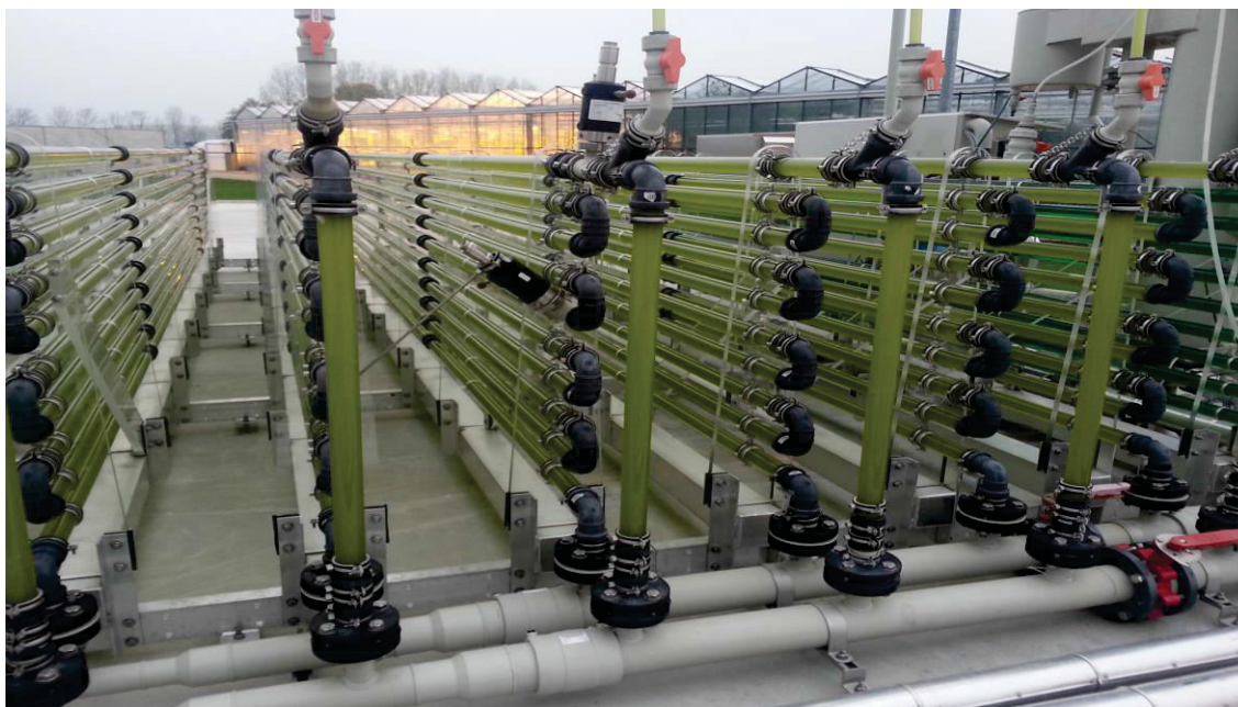
Figure 4: Photograph of a Horizontal Tubular Reactor (HTR) (taken in November 2013; AlgaePARC, Wageningen University). HTRs are composed of horizontal transparent glass or plastic (polyethylene) tubing. Gas transfer takes place in the tube connection or via a dedicated gas-exchange unit, and the angle toward sunlight is particularly adequate for efficient light harvesting (Carvalho et al. , 2006).
