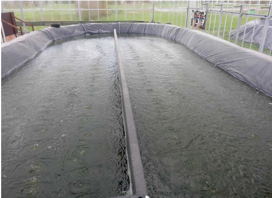
Figure 2: Photograph of a 250m 2 open raceway ponds (taken November 2013; Application Centre for Renewable Resources (ACRRES; Wageningen University initiative) in Lelystad)
