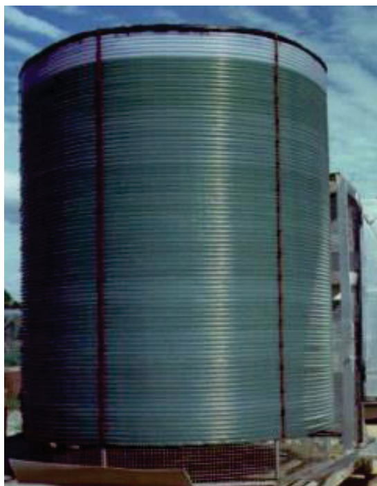
Figure 5: Helical tubular PBR (HeTRs) in Murdoch University, Australia (Chisti, 2007). HeTRs are an alternative to straight tubular reactors which are composed of a set of polyethylene tubes coiled in an open circular framework, coupled with a gas exchange tower and a heat exchange system; a centrifugal pump drives the culture broth through the long tube to the gas exchange tower (Carvalho et al. , 2006; Chisti, 2007).
