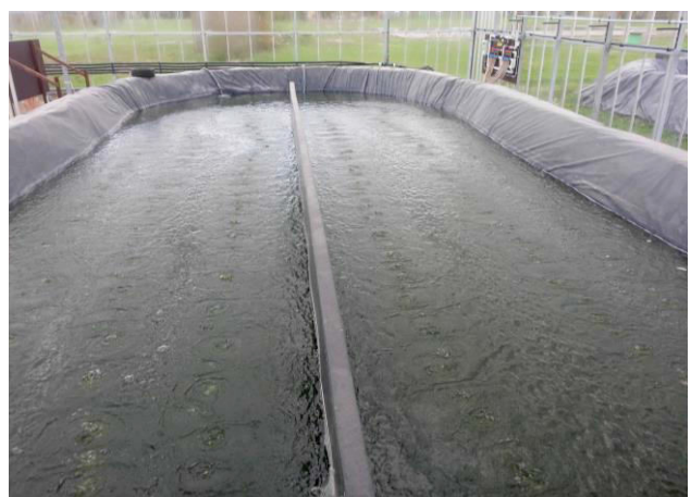
Figure 5: Photograph of a 250m 2 open raceway ponds (taken November 2013; Application Centre for Renewable Resources (ACRRES; Wageningen University initiative) in Lelystad)
