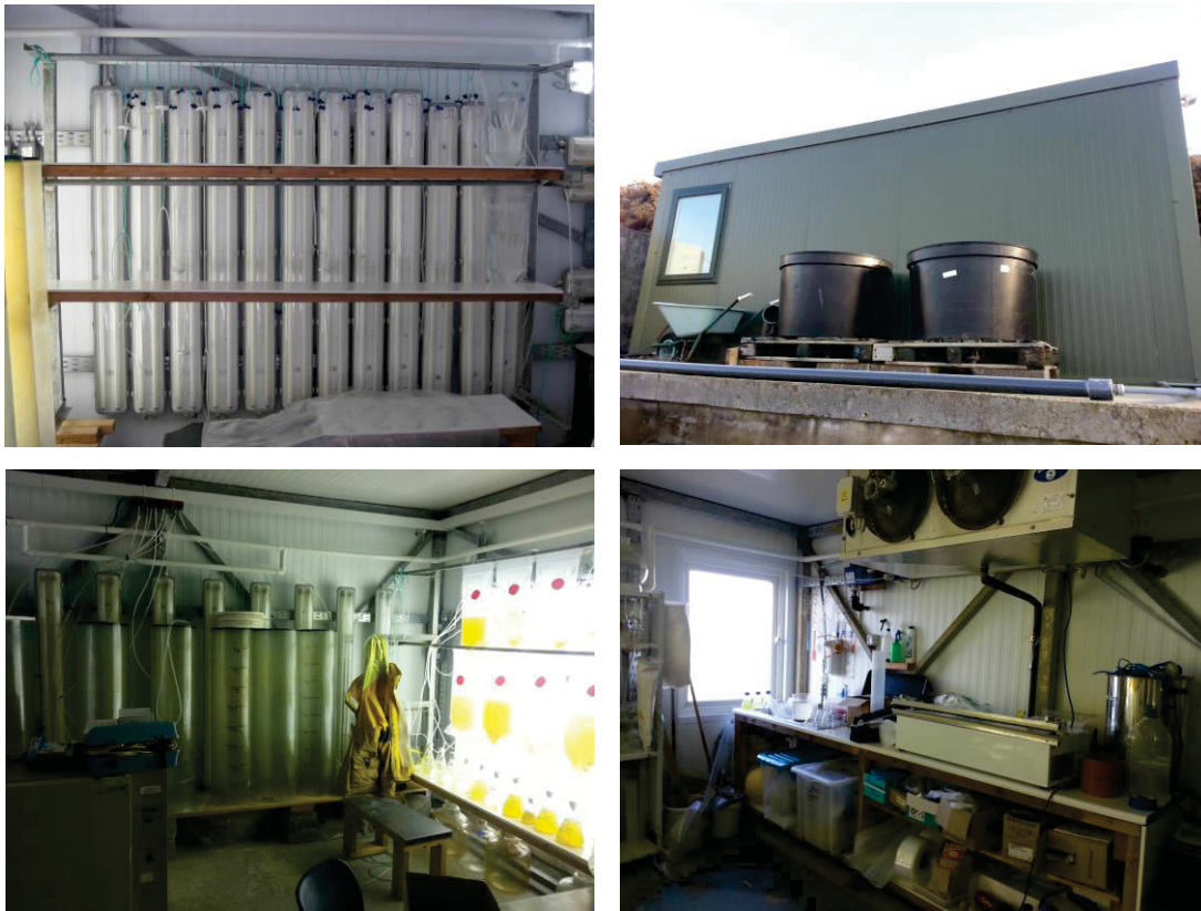
Figure 7: Photographs of 'The Shed'. Cultivation room built for a previous project, MABFUEL. Room contains a lighting panel, shelving and culturing frame (to hang bags), laminar flow unit, refrigerator for samples, a bag sealer, sink, UV water treatment system, and an air-conditioning system to control the room temperature.
