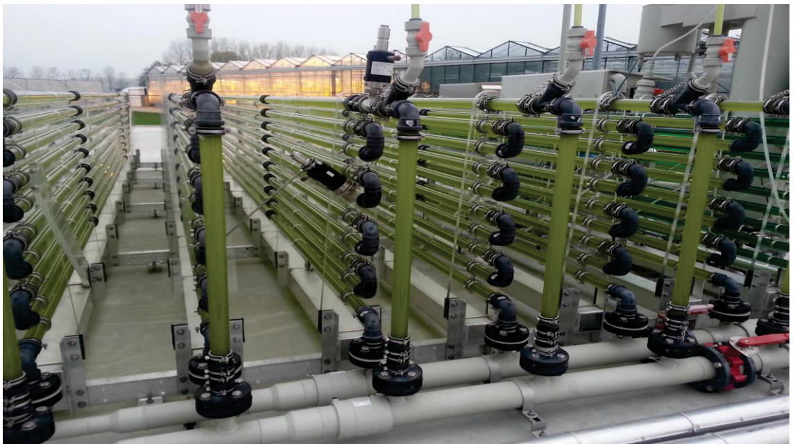
Figure 6: Photograph of a Horizontal Tubular Reactor (HTR) (taken in November 2013; AlgaePARC, Wageningen University). HTRs are composed of horizontal transparent glass or plastic (polyethylene) tubing. Gas transfer takes place in the tube connection or via a dedicated gas-exchange unit, and the angle toward sunlight is particularly adequate for efficient light harvesting (Carvalho et al. , 2006).
