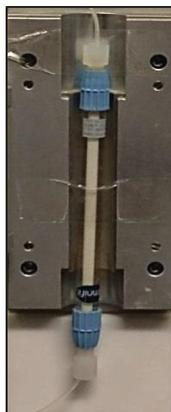
**Figure 19: Packed-bed reactor filled with 277 mg Novozyme 435 (Cal B)**
