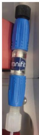
**Figure 20: Picture of an omnifit column (length: 5 cm, diameter: 3 mm) filled with 100 mg Celite-His<sub>6</sub>-AtHNL**
