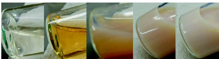
Fig. A.11. Pre-polymerization steps of pure R,F-xerogel solution (approx. 1 g) at 343 K. The first picture refers to the initial solution before heat treatment. The last one shows the pre-polymerized dispersion after 5 h.
