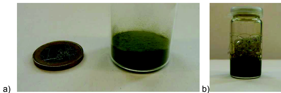
Figure 150: a) Amount of MIL101Cr-NH 2 (0.9 g) which was suspended in H 2 O (30 mL), b) suspension of 3 % MOF in 2 mL H 2 O with SDS
