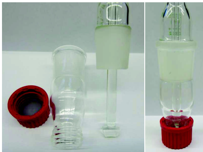
Figure 167: custom built apparatus for mixing of MOF@xerogel mixtures.
