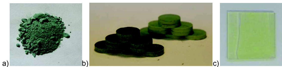
Figure 160: a) Shaping of MOF powder into b) pellets or c) as coating on glass substrates.
