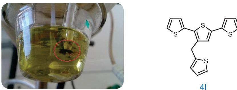
**Figure 6:** Electropolymerisation of compound **4i** at 2 V in dichloromethane (room temperature).
