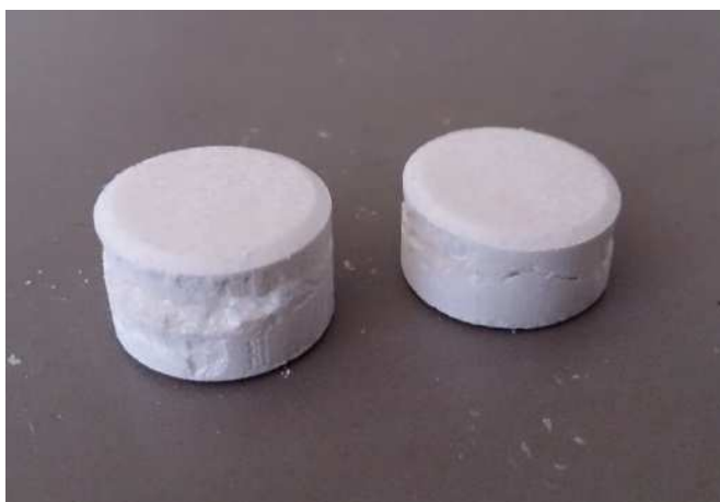
Figure 4.53. Lamination of tablets produced with Parateck® ODT
