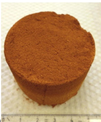
Fig. 22. (a) Molecular presentation of the polymerization mechanism of resorcinol and formaldehyde. Reprinted from ref. 203, Copyright 1997, with permission from Elsevier. (b) Photograph of a subcritically dried resorcinol-formaldehyde aerogel. Reprinted from ref. 204, Copyright 2014, with permission from Elsevier.
