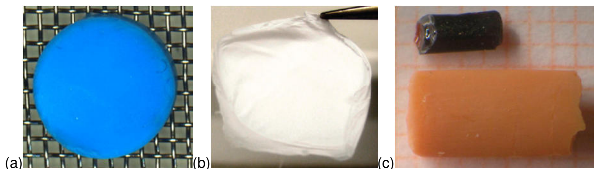
Fig. 24. (a) Photograph of monolith silica aerogel Cu-BTC composite. Reprinted from ref. 211, Copyright 2012, with permission from Elsevier. (b) Photograph of ZIF-8@PVP (PVP = polyvinylpyrrolidone) fibers. Reproduced from ref. 215, Copyright 2011, with permission of The Royal Society of Chemistry. (c) Photograph of phase, pure 'MIL-100(Fe)-like' monoliths, which were air-dried (top) and supercritically dried with \text{CO}_2 (bottom). Reproduced from ref. 218, Copyright 2009, with permission of The Royal Society of Chemistry.
