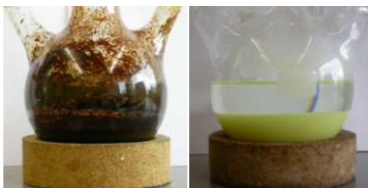
Fig. 9.1.7.1: The reaction flask after synthesis of N,N' -dimethylacetamide azine dihydrochloride by using \text{SOCl}_2 (left) or \text{POCl}_3 (right).
