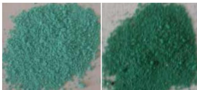
Fig. 6.4.1.15: Sample images of 33 as synthesized (as) measurement (blue, left) activated (act) measurement (dark green, right).
