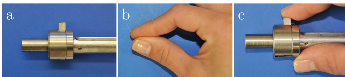
Figure 30: Trigger mechanism of the SDP (a), one-point pinch grip (b), and triggering of the SDP (c)
