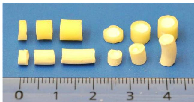
Figure 43: Doses of the wax-coated extrudates by immersion (first row) and the wax-coated co-extrudates (second row) after dissolution of 16 h in 900 mL of degassed, demineralised water at  $37.0 \pm 0.5 \text{ }^\circ\text{C}$ , displayed scale in cm
