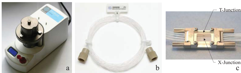
Figure 2.4: Mitos P-Pump (a), Flow Resistor F1 (b), and Droplet Generator Connection with T- and X-junction (c). Pictures are taken from dolomite website.
