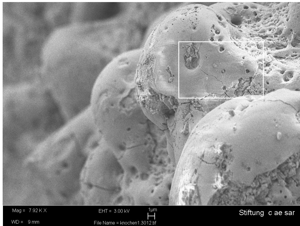
Figure 5.9.a: Laser incision in ethanol dehydrated bone, 64 laser passes ( N_{eq} = 73 ) (irradiation parameters as described in chapter 5.1), view of the incision sidewall and bone surfaces
