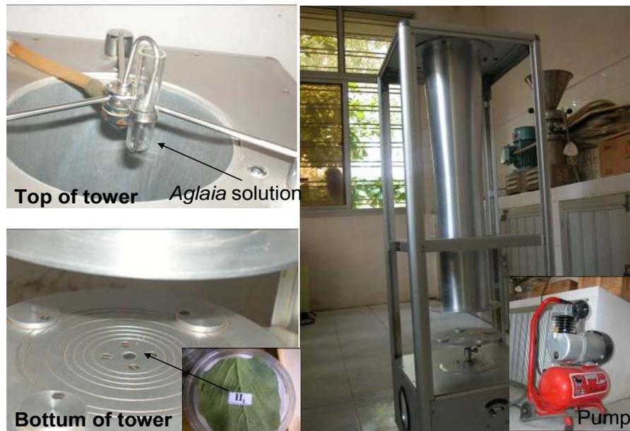
Fig. 2.1 Potter spray tower used to spray *Aglaiia* solution
