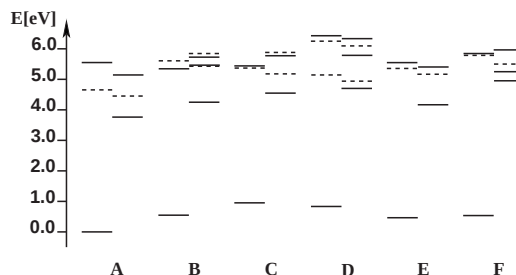
Fig. 10. Relative DFT/MRCI energies (TZVP basis) of low-lying electronic states for various tautomers of uracil: diketo (A), ketoenol (B)–(E), dienol (F) ( cf. Fig. 1). Solid lines denote states of A' symmetry, dashed lines A'' states. For each tautomer, singlets are shown to the left, triplets to the right.
