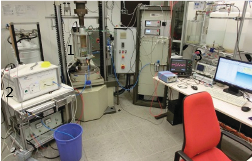
Figure 4.1: Sound transmission setup with the triaxial compression cell. Compression cell (1), pressure control with a force loading mechanism (2), and measurement chain with sound wave generator and receiver (3).
