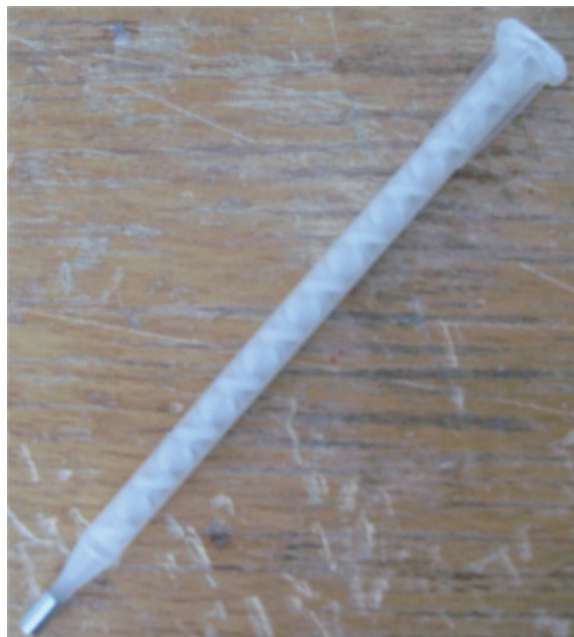
Figure 2.3: Mixing nozzle: plastic tube containing an interrupted helical particle rotating device. The tube has a length of \approx 200\text{mm} and a diameter of \varnothing \approx 6\text{mm} .
