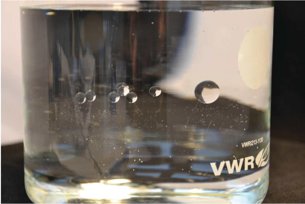
Figure 3.9: PDMS spheres imbedded in a diffusion layer of H_2O+NaCl during the hardening process. Seven spheres with a diameter of \varnothing 6mm and one sphere with a diameter of \varnothing 13mm are visible.
