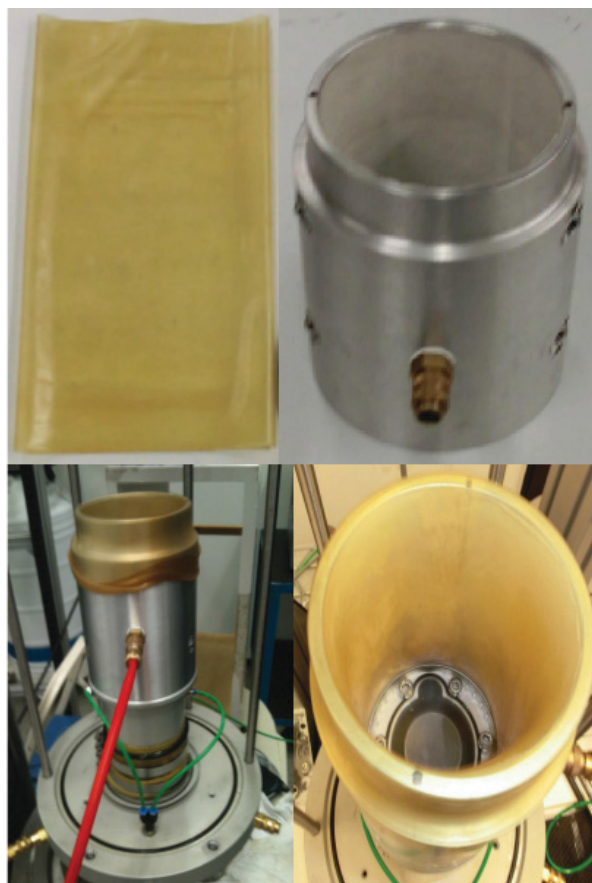
Figure 4.6: Picture series to visualize the latex membrane stabilization. Upper left: latex membrane with a height of 200mm, a diameter of \varnothing 100\text{mm} , and thickness of 1mm. Upper right: aluminum cylinder with vacuum connection in the middle. Lower left: installed and vacuum sealed latex membrane with aluminum cylinder on top of the ultrasonic transducer. Lower right: latex membrane pressed on the inner aluminum cylinder surface due to evacuation, the ultrasonic transducer is visible on the bottom.
