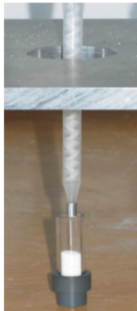
Figure 2.4: Mixing nozzle outlet with the sample cell.
