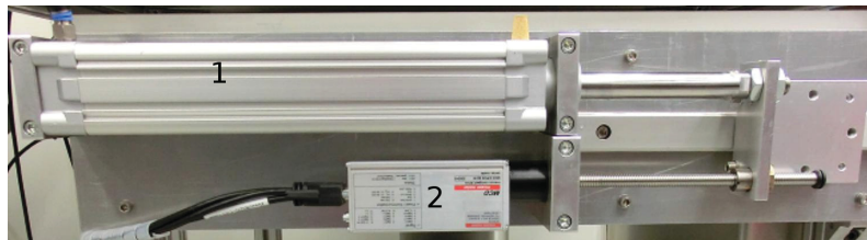
Figure 4.3: Pressure control for generating triaxial compression. (1) DNC-50-250-P-S11 cylinder from the Festo ® company and (2) a stepper motor MCD EPOS 60 W from the Maxon ® company
