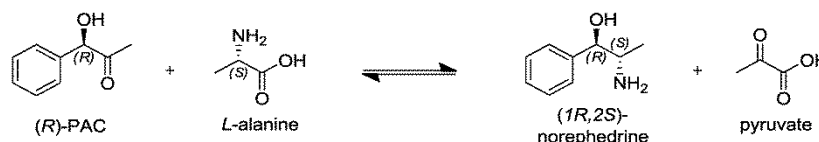
Scheme 2: Reaction equilibrium determined for the reaction of PAC+alanine to norephedrine and pyruvate
